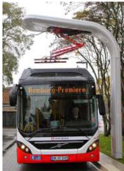
Figure 7 – Volvo and Siemens overhead charging system in Hamburg Germany
