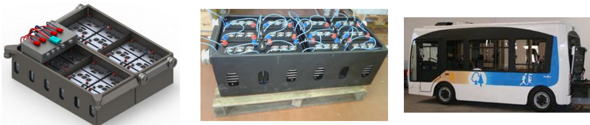
Figure 13: Design (left) realization (middle) and installation (right) of the battery system
