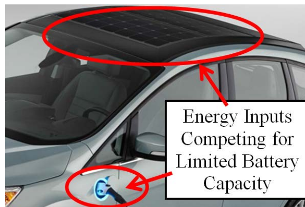
Figure 1: Roof-installed PV panels provide slow trickle charging compared with the much faster grid-sourced power. If these both feed the same battery then the grid-charging may effectively negate future solar generation later in the day.
