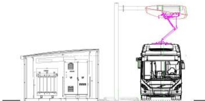
Figure 5: Rapid charging system – a potential universal charger option and overhead interface connector (Courtesy of Siemens)
