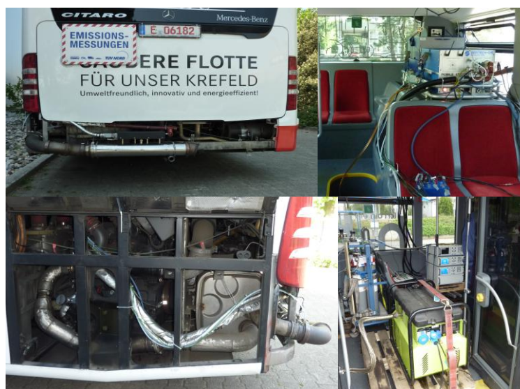
Figure 1: Analyzer systems inside and measurement pipes outside the vehicle
