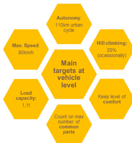
Figure 4: Vehicle main targets considered in the electrification process
