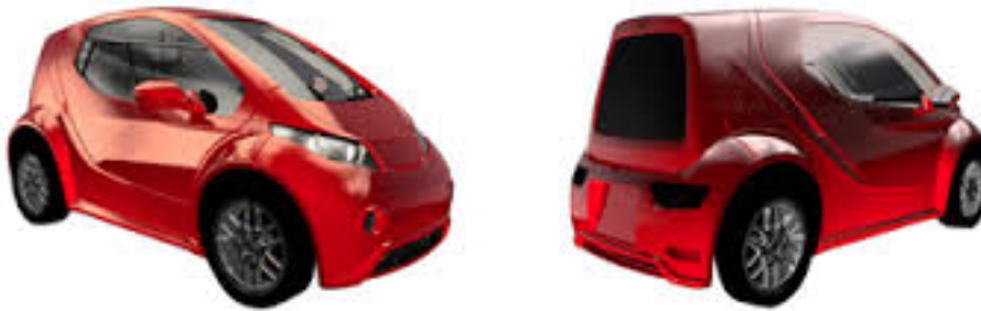
Figure 5: IMA Colibri electric one-seater with full passenger car safety and highway capability, expected to hit the German market in 2016
