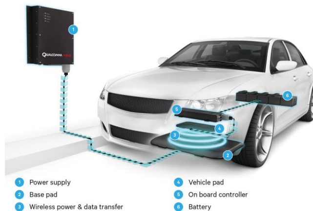
Fig. 1: Wireless electric vehicle charging (WEVC) system components.
