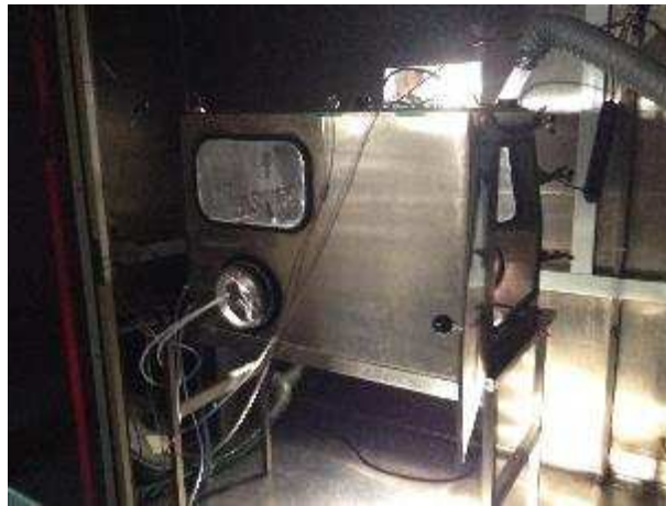
Figure 3 The glove box (0.38 m 3 ) located in the test room (65 m 3 ).
