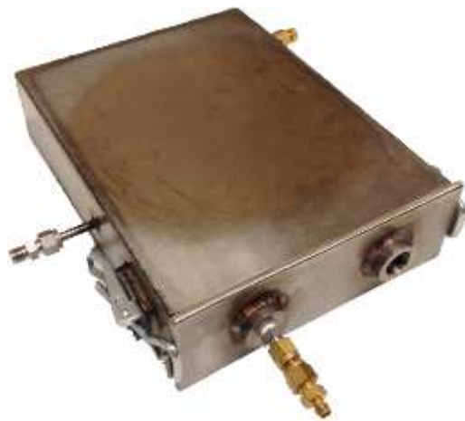
Figure 2 The battery cell was placed inside the battery box that has connections for inflow of nitrogen and an opening in the lid for the outflow. The lid also carried connections for temperature and pressure probing of the box's inside.
