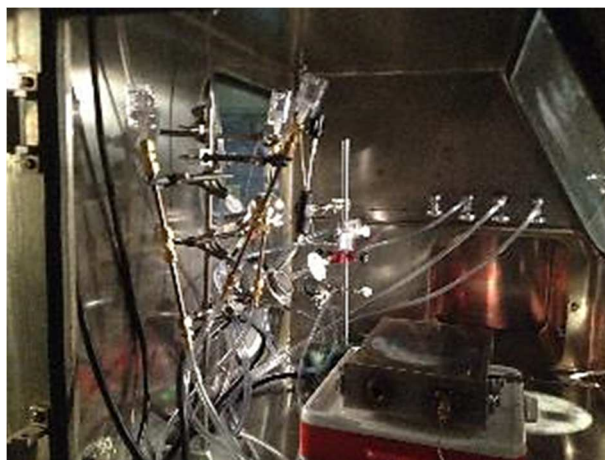
Figure 4 Inside the glove box with all sampling equipment setup and the battery box on the heat source.
