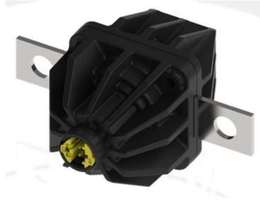
Figure 4 The heavy-duty PSS-4/NC has a max rated voltage capacity of 600 VDC under resistive load, and under inductive load it is specified for a max switching capacity of 8000 \text{ A} / 450 \text{ V} / L/R 0.5 \text{ ms} time constant. [3]
