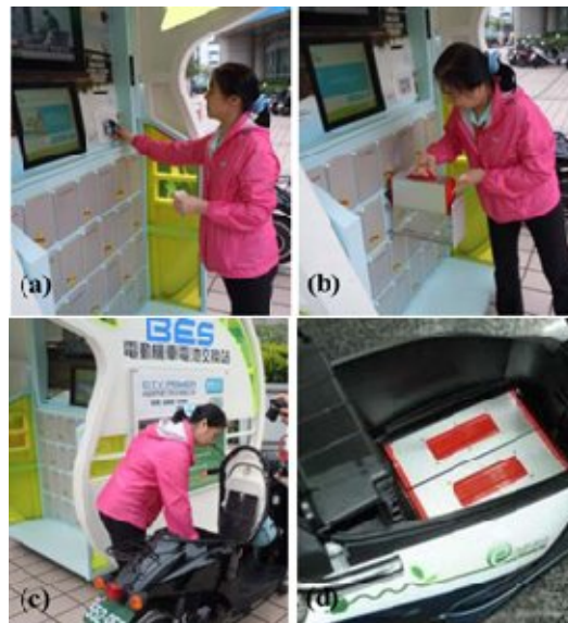
Figure 3: The battery swapping procedure at a station
