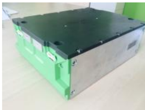
Figure2: Basic ICPT LTO module with 12S2P configuration
