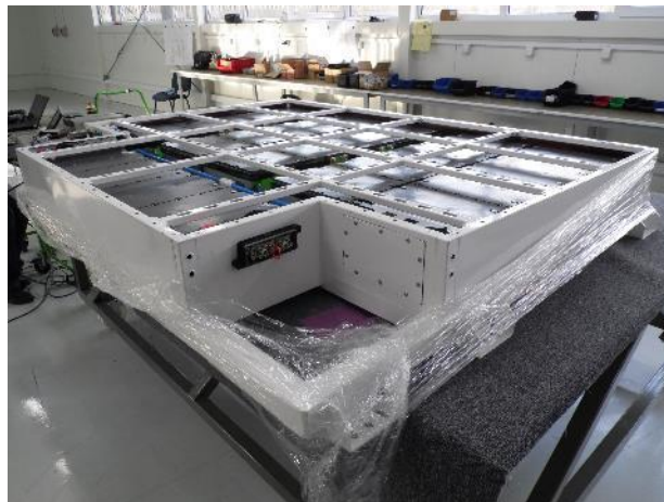
Figure3: Example of flat ICPT LTO battery pack roof mounted
