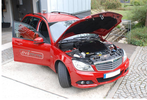
(a) Test vehicle EVA-MRM, an all-wheel driven electric passenger car
