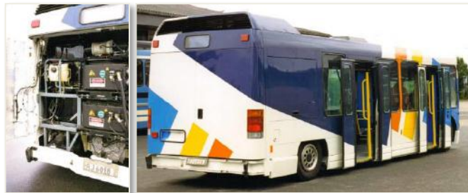
Power pack for hybrid bus demonstration (1995)
