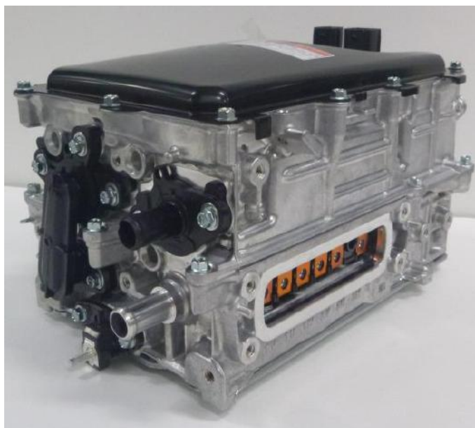
Power Control Unit
