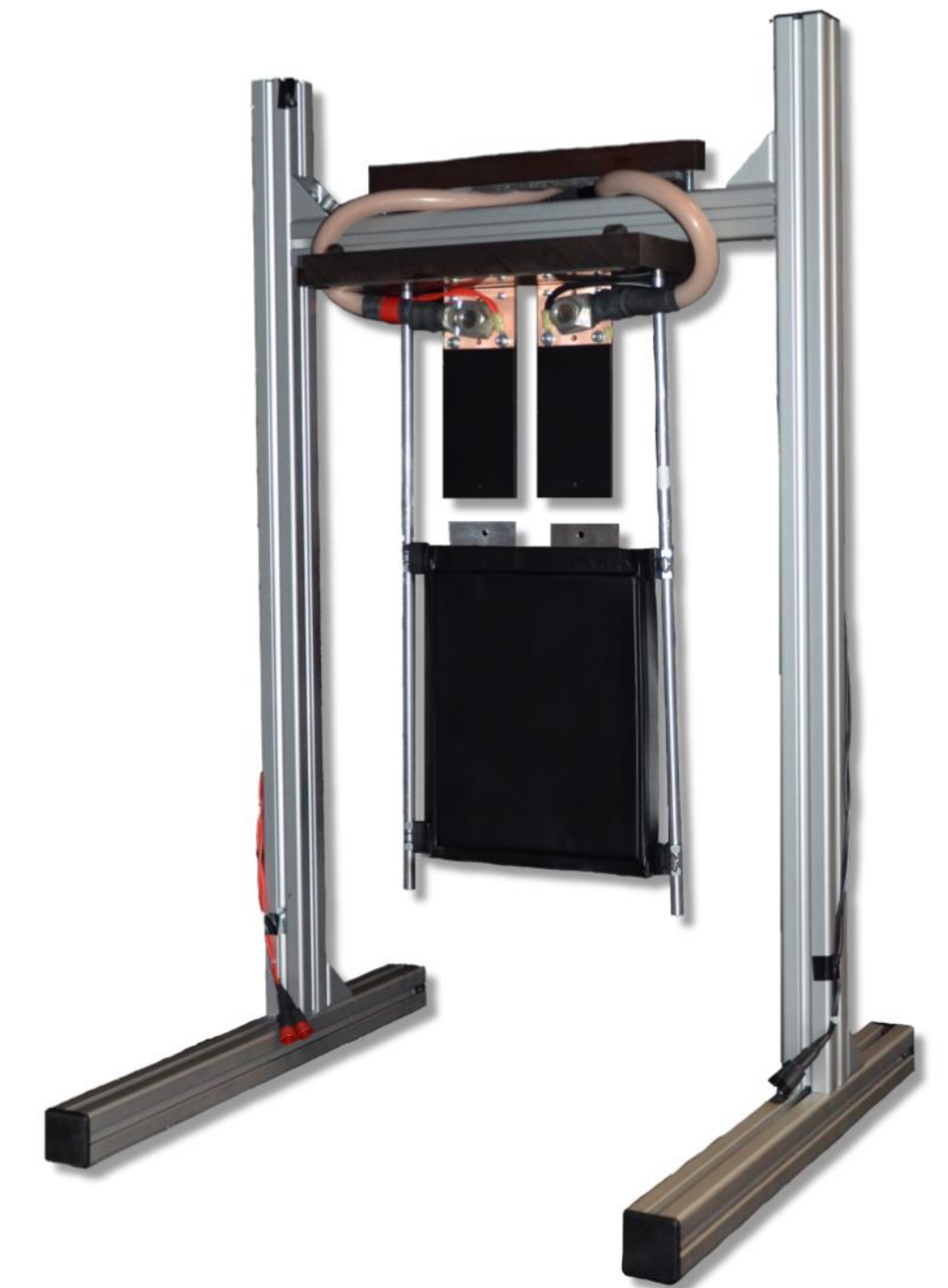
Experimental 40 Ah pouch cell with connectors
